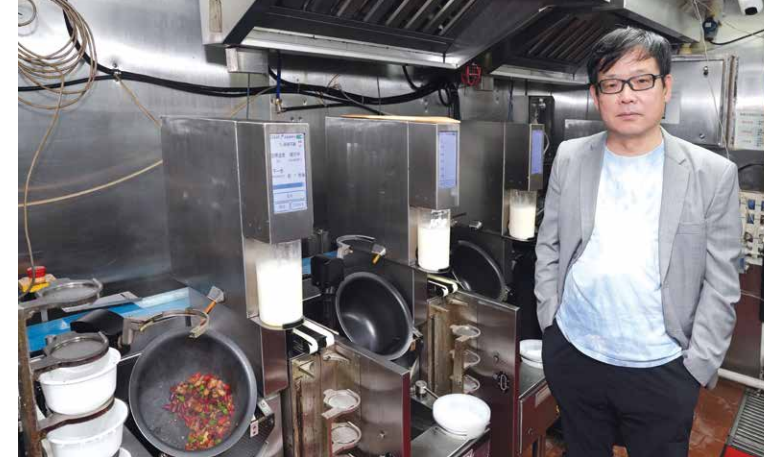
Combining stir-frying, mixing, and precision heating techniques, the multicooker developed by Professor Chen Guanhua and his team can quickly and efficiently prepare and plate up food. (Courtesy of Hong Kong Economic Journal)
