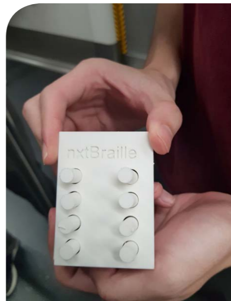
The prototype of the braille keyboard and reader developed by Sidhant Gupta and his teammates.
