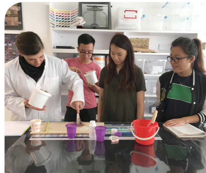
One group mixing lime plaster with red pigment and brick powder in the laboratory to compare the visual differences between these stained plaster dummies in comparison with the plaster at Pun Uk.
