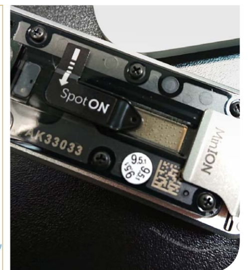
The miniaturised MinION® single molecule sequencing device used in the paper for reading out DNA.
