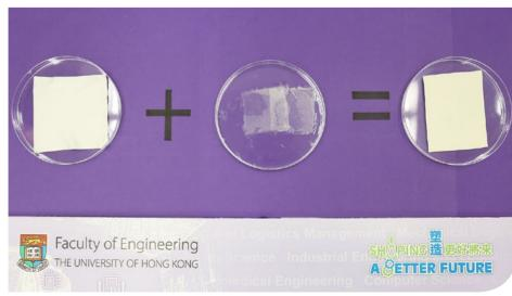
A piece of ordinary cloth (left) can become liquid-repellent (right) simply with a layer of porous surface material (middle).
