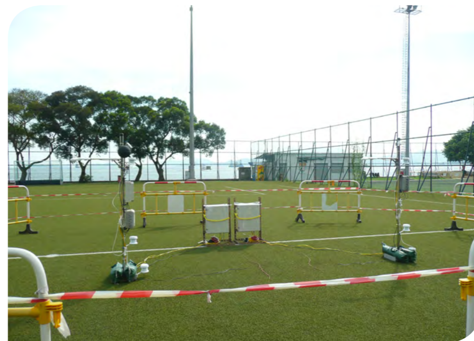
The microclimatic sensors and dataloggers installed at the field at HKU’s sports centre for the artificial turf study.
