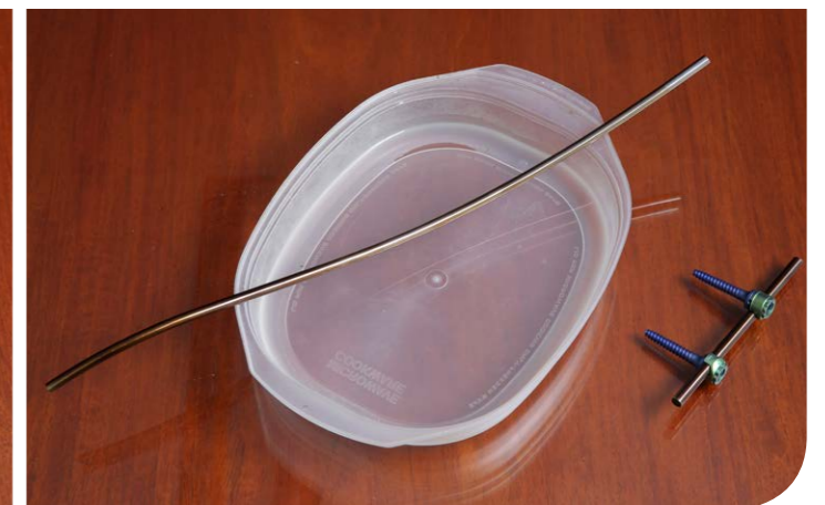
The spinal rod is made of a shape-memory alloy material that can change form. When cooled it can be bent (left) but when warmed it returns to its original shape (right).
