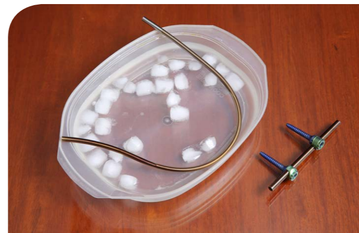
The spinal rod is made of a shape-memory alloy material that can change form. When cooled it can be bent (left) but when warmed it returns to its original shape (right).
