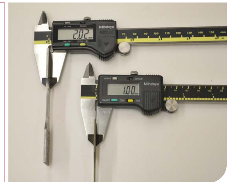
The new generation of automobile steel (right) is only half as thick (1.00mm) as the steel now used in automobiles (left, 2.02mm), while offering the same strength and ductility.
