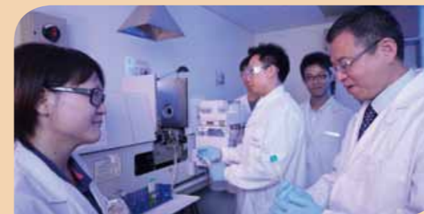
The School of Chinese Medicine uses the technique of atomic absorption spectroscopy to conduct experiments on quantitative determination of heavy metals (arsenic, cadmium, lead and mercury) contained in proprietary Chinese medicines.
