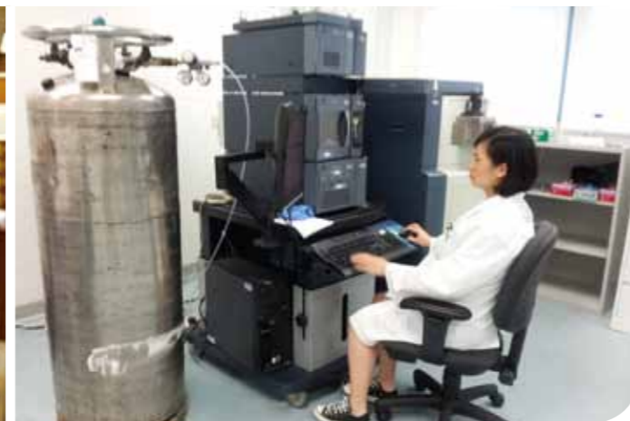
Application of advanced technologies facilitates the study of traditional Chinese medicine at HKU. The Department of Chemistry uses high performance liquid chromatography-tandem mass spectrometry (quadrupole time-of-flight) for chemical analysis of Chinese medicines and drug discovery.
