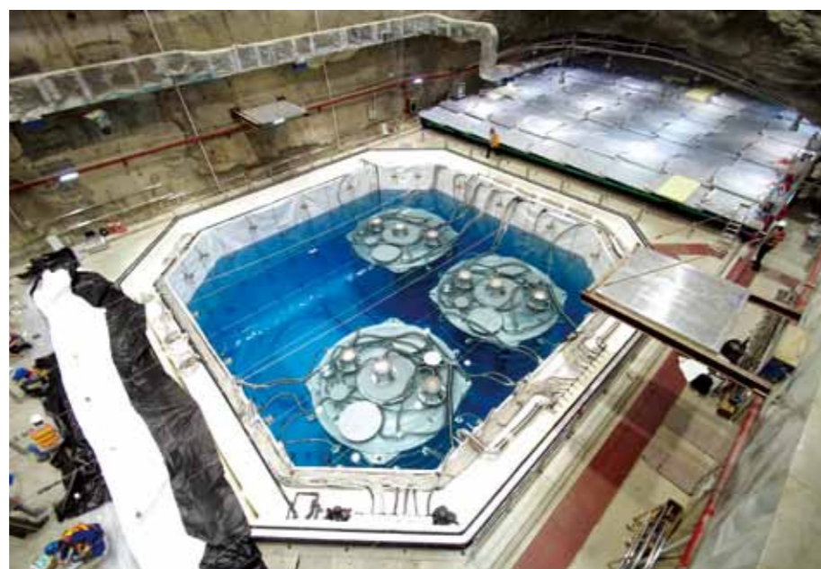
The three anti-neutrino detectors, 5m tall by 5m diameter each, submerged in pure water inside the Daya Bay Hall
