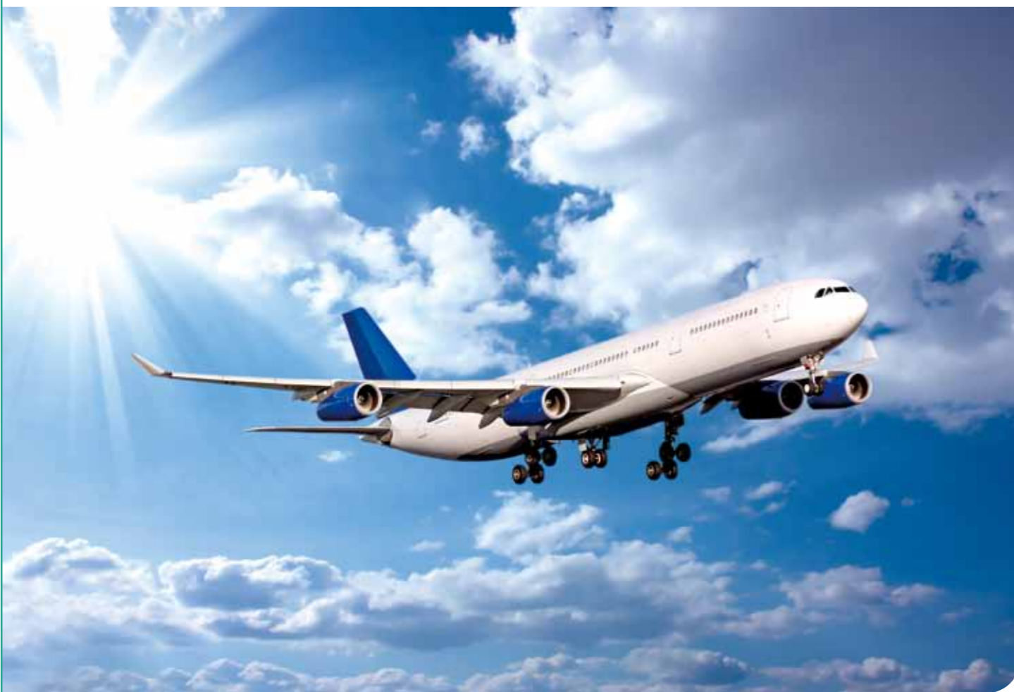
The main sources of noise are found in the turbofan engine, fuselage, high-lift wing devices, and landing gears.
