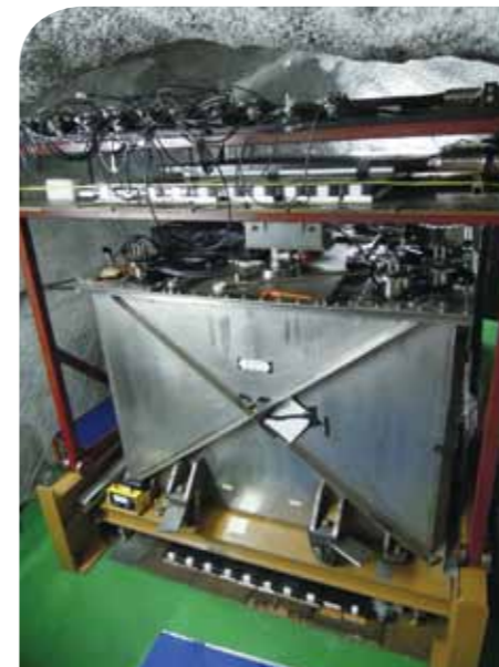
Experimental detector installed inside the Aberdeen Tunnel Laboratory
